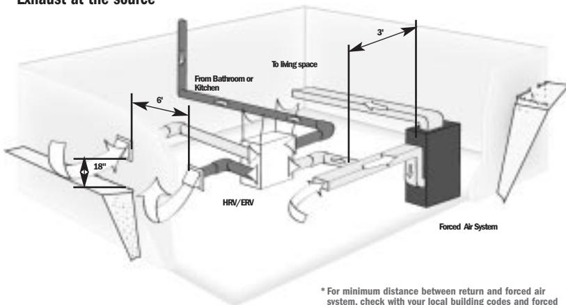
\* For minimum distance between return and forced air system, check with your local building codes and forced air system manufacturer.
