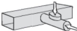
A Breathing Tee is a ventilation air supply duct with an open tee located before the connection to the return air duct. It allows the HRV to function without supply air flow rates being affected by the forced air system's fan speed.
