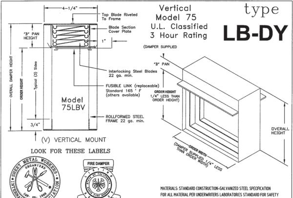
UNDERWRITERS LABORATORIES (UL555) CLASSIFIED FIRE DAMPERS. FIRE RESISTENCE RATED 3 HOURS. FOR USE IN UL CLASSIFIED BUILDING MATERIALS RATED 4 HOURS OR LESS.
