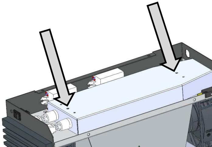
5. Remove the two (2) nuts securing the lamp cover to the chassis.
