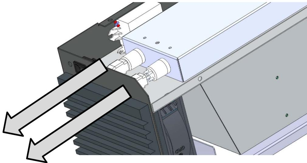
4. Gently remove the four-pronged plugs from both lamps by sliding straight off.
