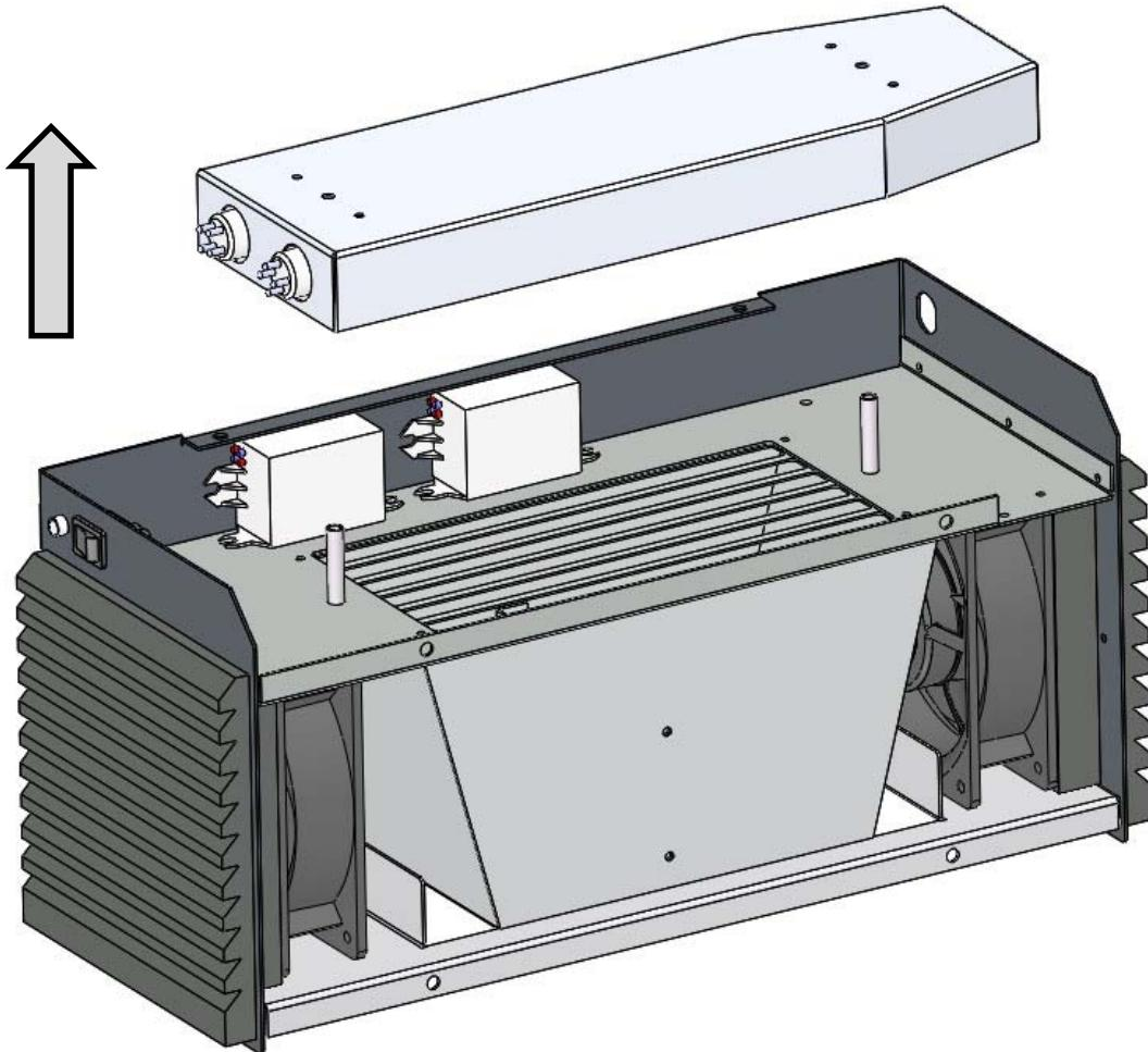
6. Remove the lamp cover assembly from the chassis.
