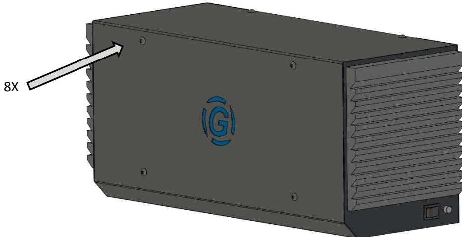
2. Remove the eight (8) cover screws using an 8/32" Allen wrench.
