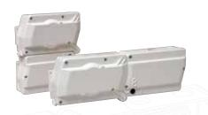
D4120W Watertight photoelectric duct smoke detector 4-wire; 100-4,000 ft/min; -4° to 158° F (-20° to 70° C); NEMA 4; 24 VAC/DC or 120 VAC; 65mA max. at 24 VDC; 2 Form C Auxiliary
