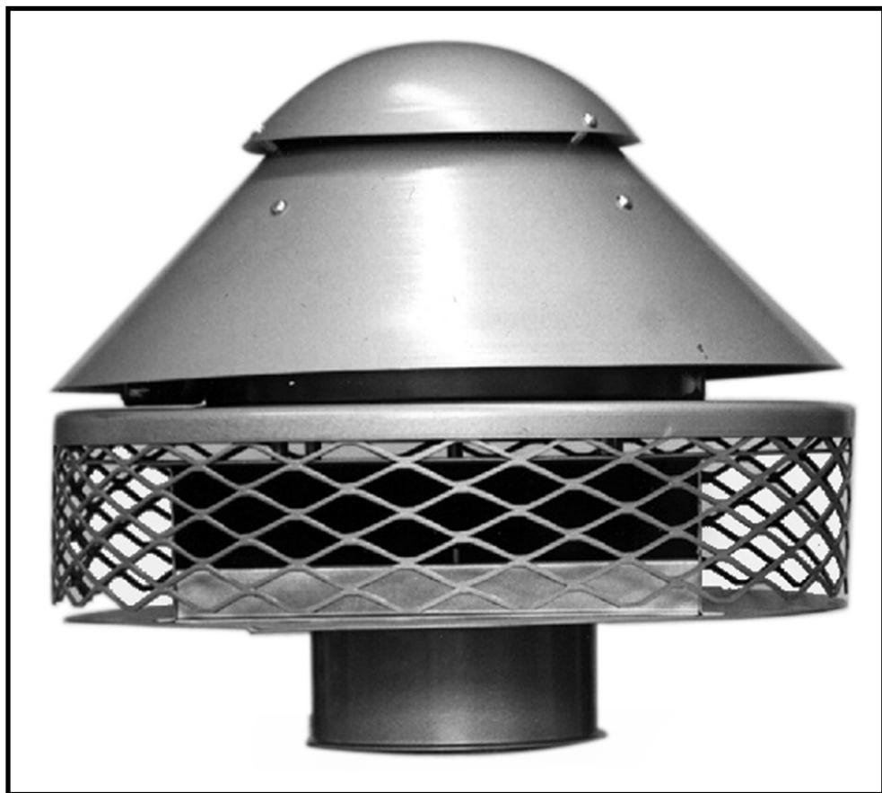
The Type "C" Chimney Top Draft Inducer is designed for installation on smoke pipes, Type "B" vents, Type "L" vents and factory built Class "A" chimneys. The Type "C" Draft Inducer is installed on the top of the vent system outside of the building.
