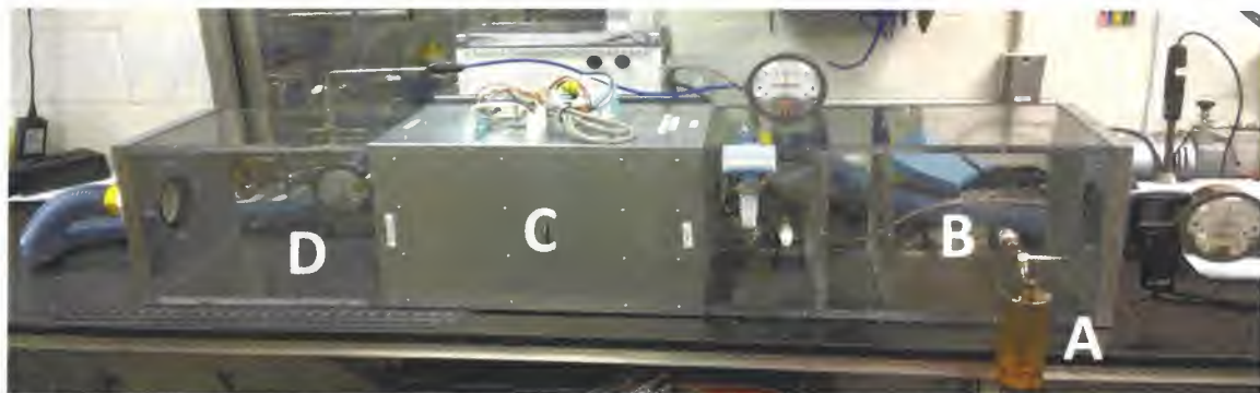
Set up demonstrating (A) Collision nebulizer aerosol generator, (B) Prechamber, (C) Test Unit containing ultraviolet photolytic unit and HEPA filter, and (D), Postchamber.
