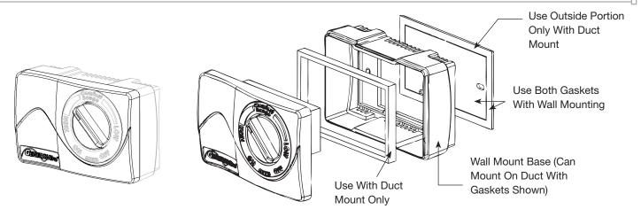
6. MHX3C: Mounting On The Return Air Duct
